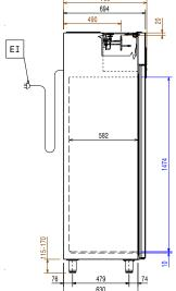
Electrical inlet (power) Refrigerant Inlet RO Refrigerant Outlet
